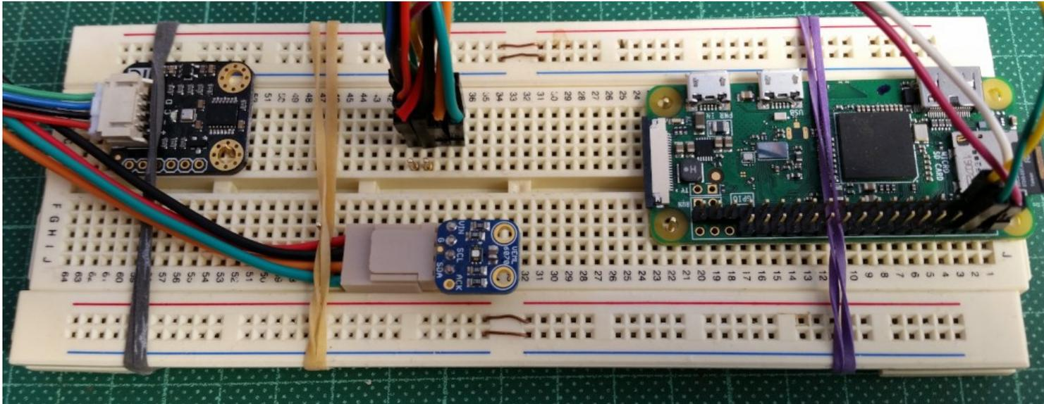
There are two breakout boards with sensor chips connected to this Raspberry Pi Zero W with Raspbian Buster installed. From left to right:
