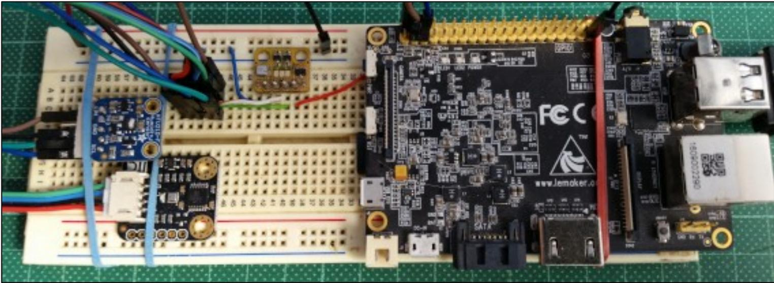
There are three breakout boards with sensor chips connected to this Bananapro with Slackwarearm installed. From left to right:
